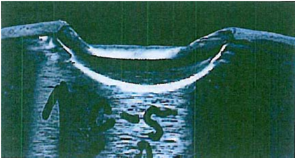
5 Severe double seam dent plate fracture.
